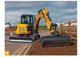
Damage can occur on site so we've fitted flat side glass windows to the 65R and 67c to minimise replacement costs.
